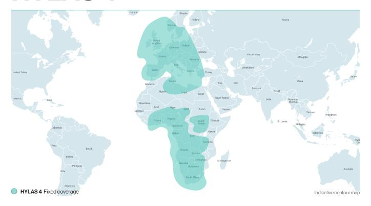
Launched in April 2018, HYLAS 4 doubles our capacity over EMEA. Using the latest Ka-band technology, it has 64 fixed beams serving Africa and Europe, as well as four independent steerable beams able to be steered anywhere visible on the Earth's disk from 33.5° W.
