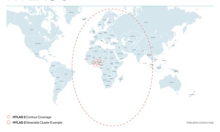
Launched in August 2019, HYLAS 3 is a steerable cluster of 8 beams that can be steered to anywhere within the 31° E coverage zone, providing flexible and high throughput connectivity across EMEA and part of Asia.
