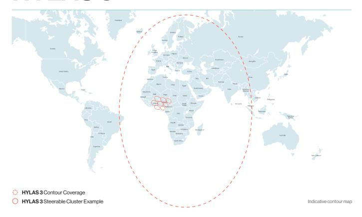
Launched in August 2019, HYLAS 3 is a steerable cluster of 8 beams that can be steered to anywhere within the 31° E coverage zone, providing flexible and high throughput connectivity across EMA and part of Asia.
