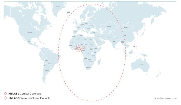
Launched in August 2019, HYLAS 3 is a steerable cluster of 8 beams that can be steered to anywhere within the 31° E coverage zone, providing flexible and high throughput connectivity across EMA and part of Asia.
