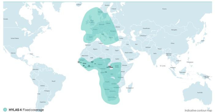
Launched in April 2018, HYLAS 4 doubles our capacity over EMEA. Using the latest Ka-band technology, it has 64 fixed beams serving Africa and Europe, as well as four independent steerable beams able to be steered anywhere visible on the Earth's disk from 33.5 °W.
