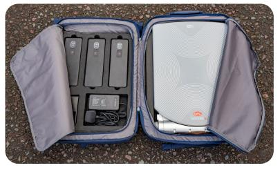
Satcube weighs just 8.6 kg and folds flat for ease of transport in most airline cabin luggage.
