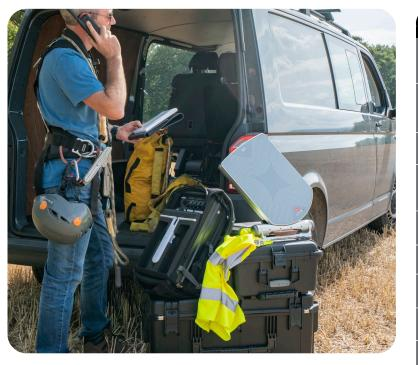
Utilising specially designed battery packs, Satcube can provide up to 3 hours transmit time. Additional batteries are available and are hot-swappable, allowing continuous operation.
